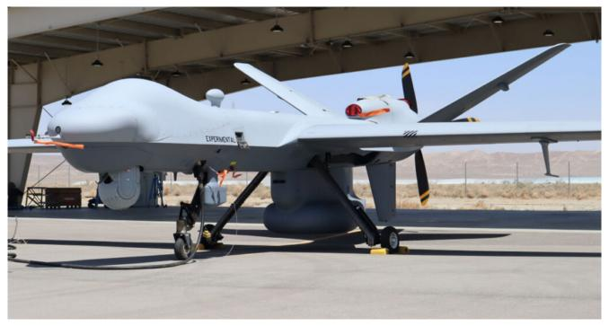
An MQ-9A Block 5 remotely piloted aircraft equipped with a Leonardo Seaspray 7500E V2 multi-mode radar. *GENERAL ATOMICS AERONAUTICAL SYSTEMS*
