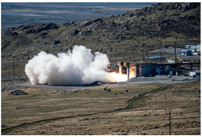
The U.S. Navy, in collaboration with the U.S. Army, conducts a static fire test of the first stage of the newly developed 34.5" common hypersonic missile that will be fielded by both services. U.S. NAVY / NORTHROP GRUMMAN
