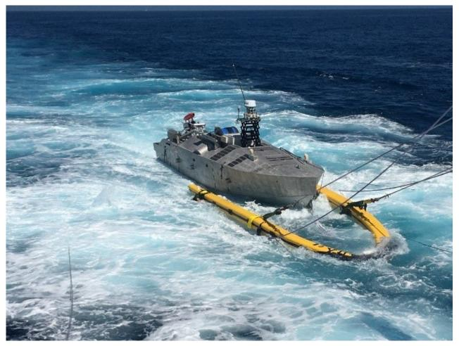
The Minecountermeasure Unmanned Surface Vehicle is recovered onboard USS Manchester (LCS 14) during Unmanned Influence Sweep System initial operational test and evaluation June 2021. U.S. NAVY WASHINGTON, D.C. – Program Executive Office, Unmanned and Small Combatants (PEO USC) announced July 28 the Unmanned Influence Sweep System, a critical component of the Navy's suite of mine countermeasure technologies, has achieved
