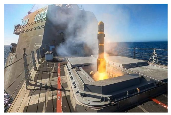
An AGM-114L Longbow Hellfire missile launches from the Surface-To-Surface Missile Module aboard Independence-variant littoral combat ship USS Montgomery (LCS 8). *U.S. NAVY / Lt.j.g. Samuel Hardgrove*
