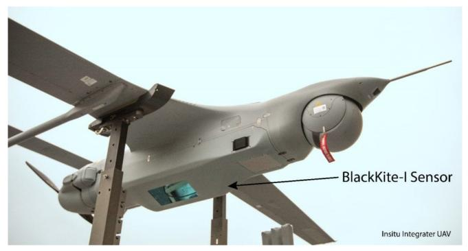
Logos Technologies LLC's BlackKite-I sensor, shown mounted on an Insitu Integrator unmanned aircraft. *LOGOS TECHNOLOGIES LLC* FAIRFAX, Va. — Logos Technologies LLC has successfully flown its wide-area motion imagery (WAMI) sensor aboard an RQ-21A Blackjack unmanned aircraft at a test range in Boardman, Oregon, the company said in a release.
