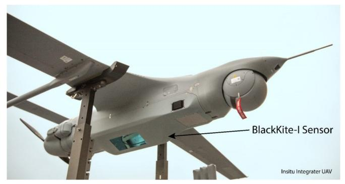
The BlackKite-I sensor on an Insitu Integrator unmanned aircraft system. *LOGOS TECHNOLOGIES*
