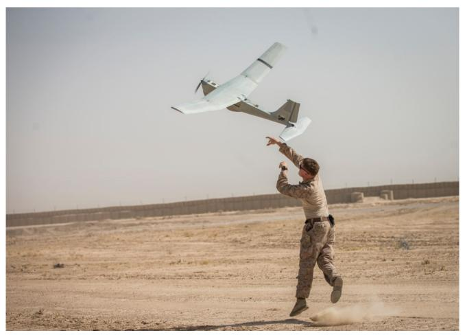
An Aerovironment Puma 3 AE small unmanned aircraft system can be launched by hand, bungee, rail or vehicle. *AEROVIRONMENT* ARLINGTON, Va. – AeroVironment Inc. received a \$6.2 million firm-fixed-price contract award for Puma 3 AE small unmanned aircraft systems and spares on May 3, for the U.S. Marine Corps, the company said in a June 14 release. Delivery is anticipated to be completed in July 2022.
