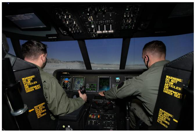
Marine Corps aviators in the CH-53K Containerized Flight Training Device (CFTD) experience a highly immersive virtual environment allowing flight crews to train on the full scope of Marine Corps heavy lift missions, including external lift operations. U.S. MARINE CORPS
