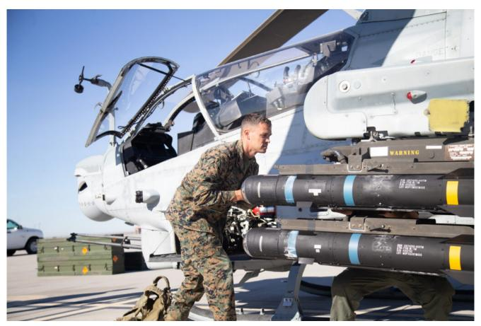
U.S. Marine Corps Chief Warrant Officer 3 Michael Brawn, aviation ordnance officer, Marine Operational Test and Evaluation Squadron 1 (VMX-1), loads a joint air-to-ground missile onto an AH-1Z Viper during an operational test at Marine Corps Air Station Yuma, Arizona, Dec. 6, 2021. U.S. MARINE CORPS / Cpl. Gabrielle Sanders
