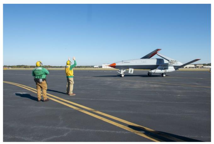
The U.S. Navy and Boeing conducted ground testing of the MQ-25 Stingray at Chambers Field onboard Naval Station Norfolk, Virginia. The MQ-25 Stingray is an unmanned aerial refueling aircraft. U.S. NAVY / Mass Communication Specialist 2nd Class Sam Jenkins
