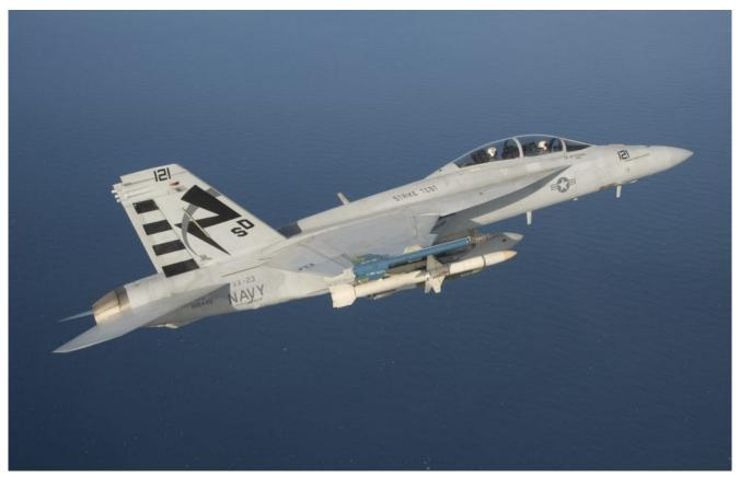
A 2012 photo of an F/A-18F Super Hornet assigned to the Salty Dogs of Air Test and Evaluation Squadron (VX) 23 conducting a captive carry flight test of an AGM-88E Advanced Anti-Radiation Guided Missile at Naval Air Station Patuxent River, Maryland. U.S. Navy / Greg L. Davis
