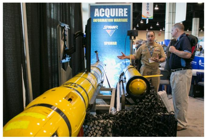
Littoral Battlespace Sensing Unmanned Underwater Vehicles (LBS-UUV) on display at the Navy League's Sea-Air-Space conference and exhibition in 2017. The LBS-UUV is made up of two vehicle types, a glider and an autonomous undersea vehicle. U.S. NAVY / Krishna M. Jackson
