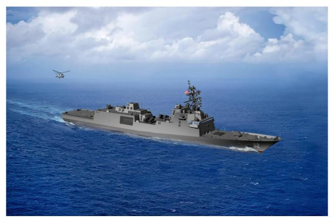
An artist's rendering of the guided-missile frigate FFG(X). The new small surface combatant will have multi-mission capability to conduct air warfare, anti-submarine warfare, surface warfare, electronic warfare, and information operations. Construction on the lead ship is set to begin in the first quarter of fiscal 2022. U.S. Navy
