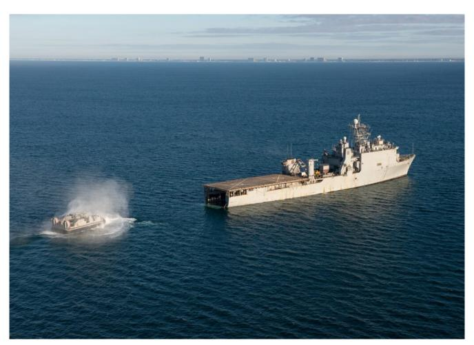
The next generation landing craft, ship to shore connector (SSC), landing craft, air cushion (LCAC), successfully completed well deck interoperability testing with the amphibious dock landing ship USS Carter Hall (LSD 50) and demonstrated the craft are another step closer to fleet integration.
