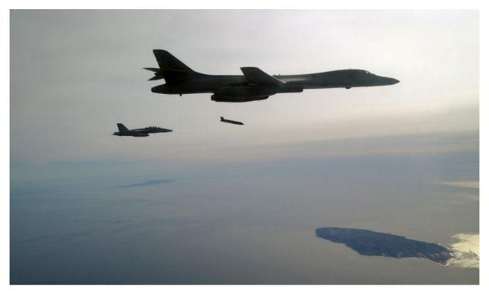
An LRASM being dropped from a B-1B Lancer bomber. *LOCKHEED MARTIN*
