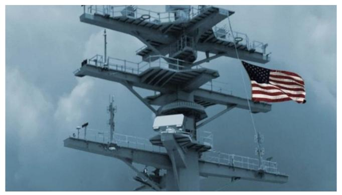
SAAB's AN/SPN-50(V)1 radar. Saab
