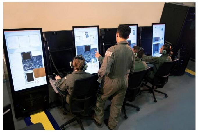
Naval aviators train on E-2D distributed readiness trainers, which are training devices capable of elements of two, five crewmember aircraft to conduct a single training scenario simultaneously and execute the full list of tactics, techniques, and procedures. *U.S. NAVY*
