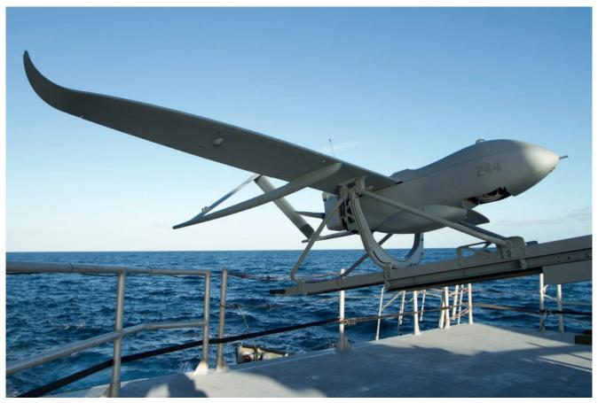
The Aerosonde UAS has been deployed on a Navy Arleigh Burkeclass guided missile destroyer in the 7th Fleet. TEXTRON SYSTEMS
