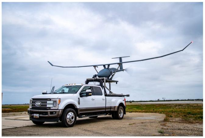
A Vanilla ultra endurance land-launched unmanned aerial vehicle (UAV) undergoes operational pre-flight checks during U.S. Pacific Fleet's Unmanned Integrated Battle Problem (UxS IBP) 21 at Naval Base Ventura County, Point Mugu. UxS IBP 21 integrates manned and unmanned capabilities into challenging operational scenarios to generate warfighting advantages. U.S. NAVY / Construction Mechanic 2nd Class Michael Schutt
