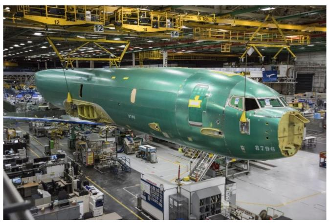
Norway's first P-8A Poseidon aircraft is moved from a rail car through the air to the first step of the assembly process, the Fuselage Systems Installation tool, in Renton, Washington. *BOEING*
