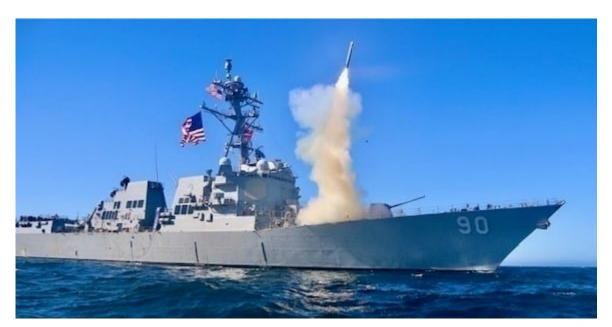
he guided-missile destroyer USS Chafee (DDG 90) launches a Block V Tomahawk, the weapon's newest variant, during a three day missile exercise. This event marked the first time a Block V Tomahawk missile was operationally tested, marking the Navy's transition to a more advanced capability for the fleet. Block V includes an upgrade that will enhance navigation performance and provide robust and reliable communications. U.S. NAVY / Ensign Sean Ianno
