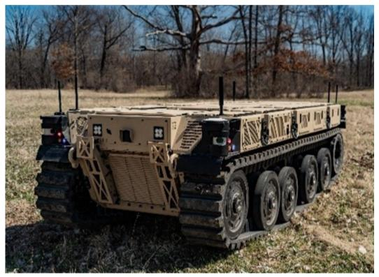
The Pratt Miller Defense EMAV can carry a 6,000-pound payload capacity and flat rack and is designed to support most logistics missions. OSHKOSH DEFENSE OSHKOSH, Wis. – Oshkosh Defense, a wholly-owned subsidiary of Oshkosh Corp., is displaying a Joint Light Tactical Vehicle and trailer and a Pratt Miller Defense Expeditionary Modular Autonomous Vehicle at the Modern Day Marine Expo 2022. The vehicles will be on display at the Walter E. Washington
