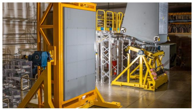
When three SPY-6(V)3 radar arrays (left) are combined, they provide 360 degree coverage for aircraft carriers, like the future USS John F. Kennedy. *RAYTHEON MISSILES & DEFENSE*NEWPORT NEWS, Va. — Raytheon Missiles & Defense has delivered SPY-6 radar arrays to the future USS John F. Kennedy (CVN 79), the first aircraft carrier to receive the advanced radar, the company announced July 18.
