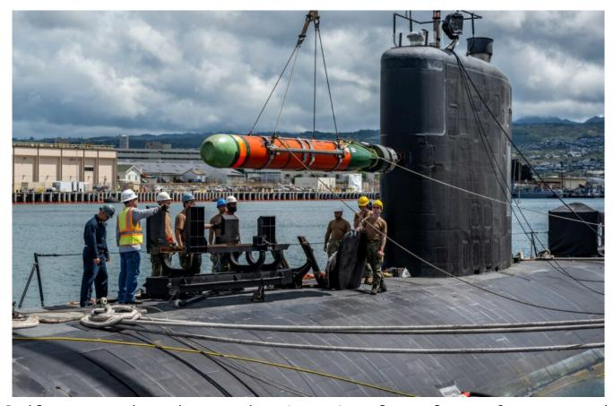
Sailors assigned to the Los Angeles-class fast-attack submarine USS Columbia (SSN 771) load a Mark 48 advanced capability torpedo for Exercise Agile Dagger 2021. *U.S. NAVY / Mass Communication Specialist 1st Class Michael B. Zingaro* ARLINGTON, Va. — The first of a new-production batch of heavy-weight torpedoes (HWTs) is slated for delivery to the U.S. Navy fleet beginning in fiscal 2022, the Navy's submarine resource sponsor said.
