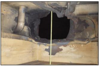
Graphic illustration and images captured by a U.S. Navy explosive ordnance disposal team aboard M/T Pacific Zircon, Nov. 16, showing the location where an Iranian-made unmanned aerial vehicle (UAV) penetrated M/T Pacific Zircon's outer hull during an attack Nov. 15. *U.S. NAVY*
