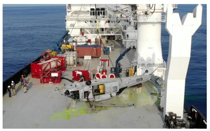
An MH-60S on deck of contracted salvage vessel off the coast of Yokosuka, Japan on March 18, 2021, having just been pulled from the depth of 19,075 feet by NAVSEA Supervisor of Salvage and Diving, (SUPSALV) at the request of the Navy Safety Center to facilitate accident investigation. NAVAL SEA SYSTEMS COMMAND
