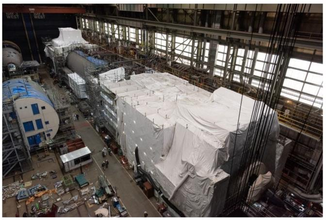
The Virginia-class submarine New Jersey (SSN 796) reached pressure hull complete in February 2021. The construction milestone signifies that all of the submarine's hull sections have been joined to form a single, watertight unit. The boat is currently 72% complete. *HII / Matt Hildreth* NEWPORT NEWS, Va. – Huntington Ingalls Industries' Newport News Shipbuilding division has achieved a milestone in the construction of the submarine New Jersey (SSN 796), the
