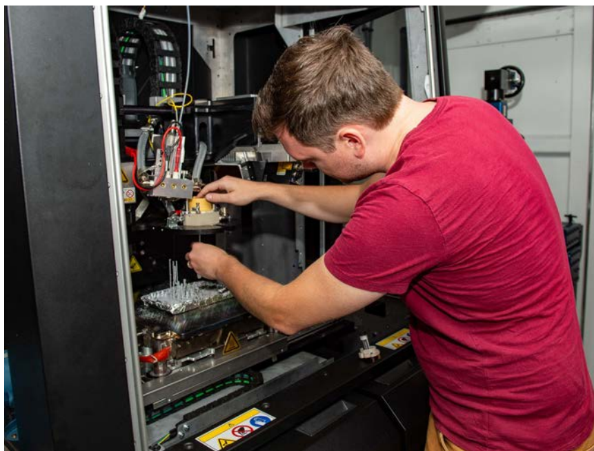
Dan Porter, a Xerox technician assembles a 3D printer head aboard Wasp-class amphibious assault ship USS Essex (LHD 2), July 9, 2022. Essex is underway conducting routine operations in U.S. 3rd Fleet.
