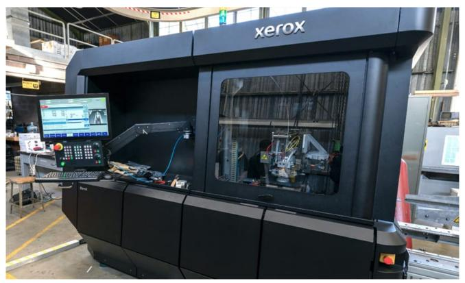
At the cutting-edge of additive manufacturing technology, this new Xerox ElemX 3-D Liquid Metal Printer is now operational in NPS' Large Experiment Annex on campus. Naval Postgraduate School
